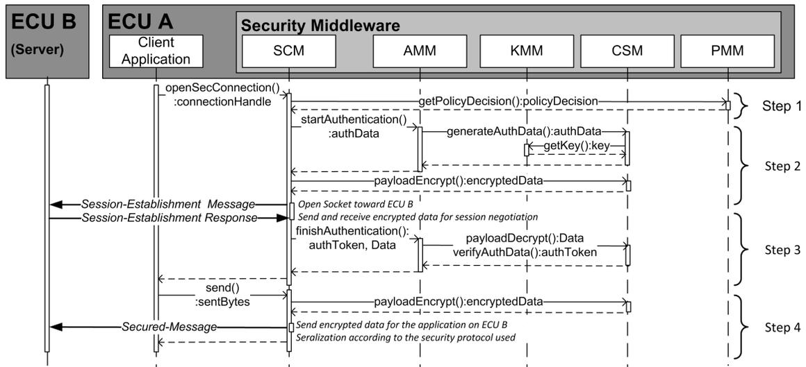
Fig. 3. Use-case: Open connection & data sending
