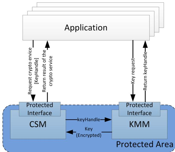
Fig. 2. Collaboration of CSM and KMM in secure environment. Keys are never communicated in plaintext outside this protected area.
