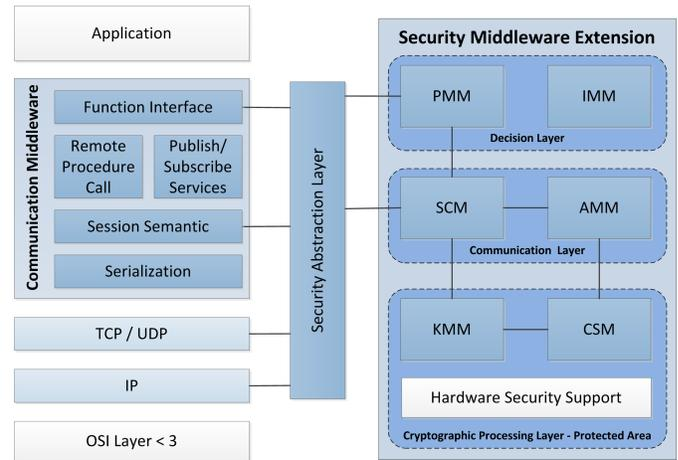
Fig. 1. Connection between Communication Middleware and Security Middleware Extension (Abbr. AMM: Authentication Management Module - CSM: Crypto-Service Module - IMM: Intrusion Management Module - KMM: Key Management Module - PMM: Policy Management Module - SCM: Secure Communication Module)
