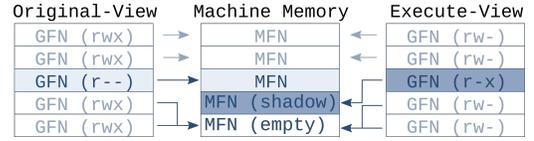
**Figure 6: The *original-view* maps the target to the original machine frame; the *execute-view* to the shadow-copy.**
