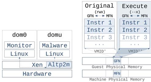
**Figure 2: Xen altp2m enables a monitor in the privileged domain *Dom0* to manage different memory views of *DomU*. While the *execute-view* maps the target guest frame *execute-only*, the permissions of the *original-view* are unchanged.**
