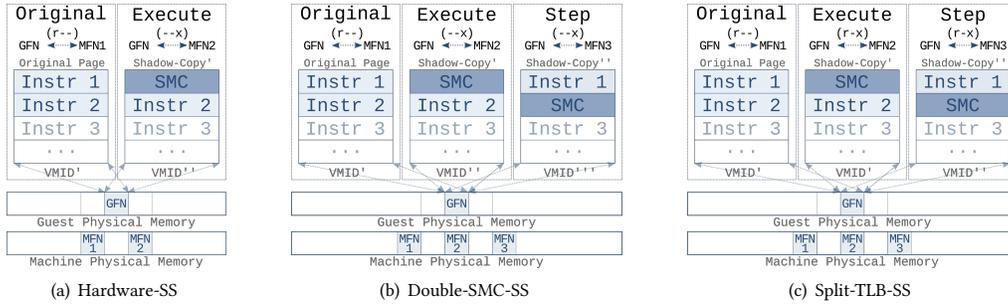
Figure 7: Xen altp2m guest-physical memory view configuration leveraging three single-stepping alternatives.
