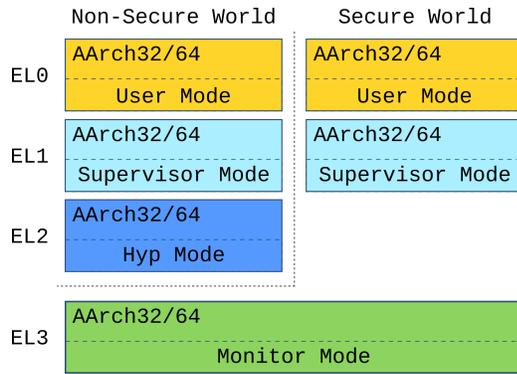
**Figure 1: Exception Level hierarchy and mode distribution on AArch32 and AArch64 until ARMv8.3. For detailed architectural differences, please refer to [1].**
