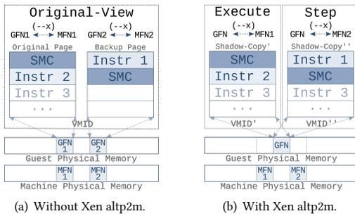
**Figure 3: On execution of the first SMC in the original page, the VMM redirects control-flow either to the backup page (a) or switches to the *step-view* (b) to single-step Instr 1. In both cases, the pages are marked *execute-only*.**
