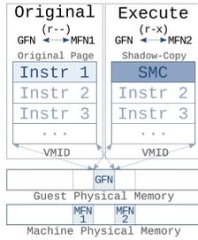
**Figure 5: The *original-view* translates the guest frame to MFN1, while the *execute-view* translates the same guest frame to MFN2. Both views are tagged with the same VMID.**
