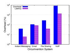
Figure 2: Overhead and latency in loading a page with different plugins.
