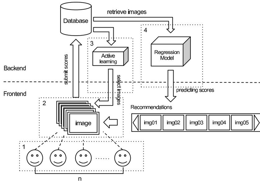
**Fig. 1.** System architecture of the OPARS. It follows the browser-server architecture. Main system modules are framed in dotted lines. They are 1) User authentication module 2) Continuous-valued rating module 3) Active image retrieval module 4) Image recommendation module.
